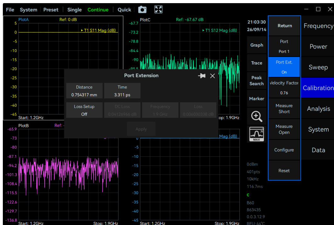
Figure 10 Port Extension Settings
