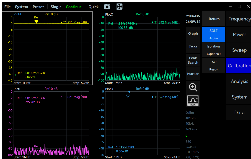
Figure 13 Creating a Marker and Performing a Local Peak Search by Double-Clicking
